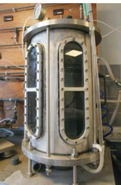
Pressure vessel used for the testing of the vertical drains (Delftse test)
